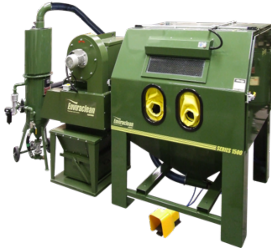
Pressure Cabinet; Dust Collector; Regrader & Blast Machine
